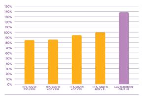
Calculations are based on an installation with the same light level, assuming typical light losses for luminaire, gear and reflection in a greenhouse.
