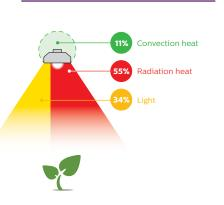
This diagram shows how the 100% of energy used by a best-in-class lighting fixture is converted into heat and light. Convection heat radiates upwards and does not affect the crop. A certain amount of energy is converted into radiation heat. High levels of radiation heat can stress or even burn the plants. LED toplighting has low levels of radiation heat, and is therefor ideal for growing cold-loving crops like lettuce and herbs, for warm dark regions and for use in low greenhouses.
